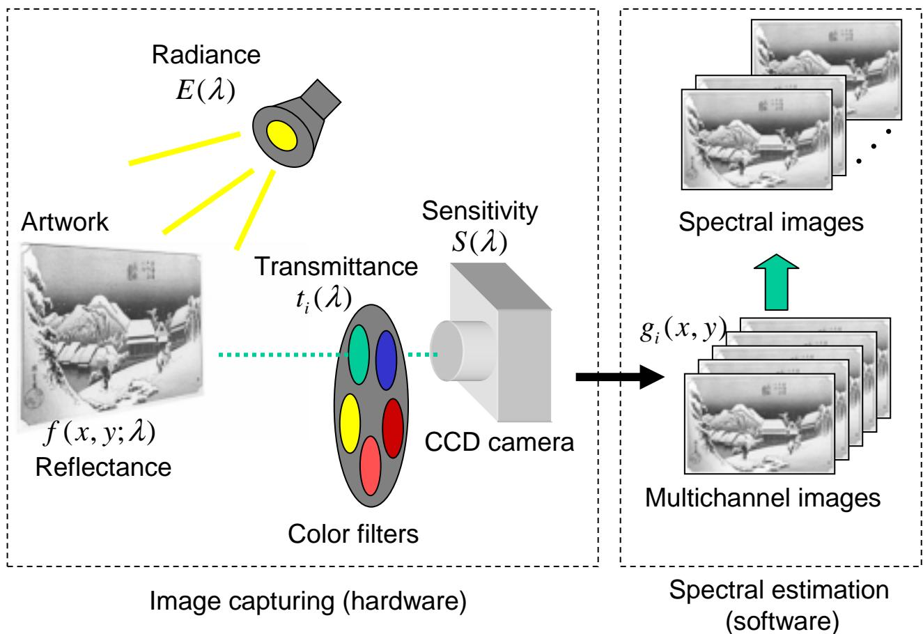
Figure 1 Multichannel imaging system.
