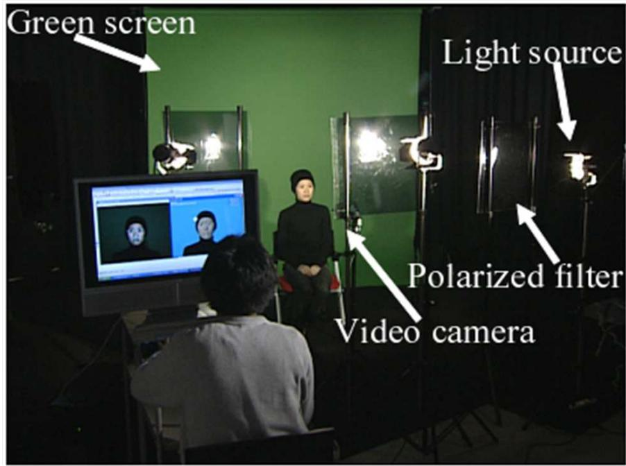
FIG.2: Geometry of a computational lighting reproduction system. The subject is illuminated by three light sources and captured by the video camera. Polarizing filters are attached in front of the light sources and the camera for removing the surface reflection on the face. The green screen is used for matting. The input images for the computational lighting reproduction process.
