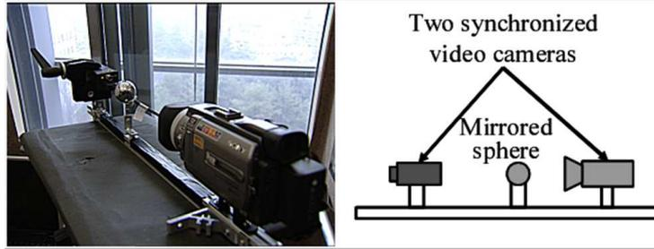
FIG.4: The camera system for capturing the background and sphere mapping video stream. In the left photo, the video camera in the foreground captures the background scene, and the other video camera captures the mirrored sphere.
