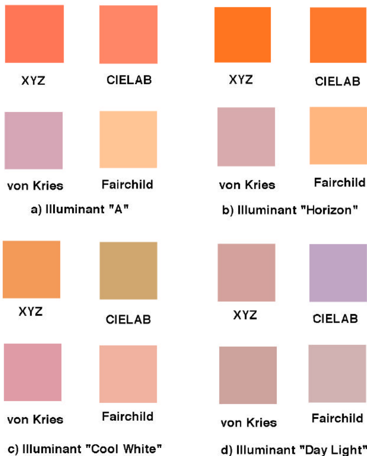
Figure 4. Predicted color appearance of skin color patches under various illuminants; (a) Prediction for illuminant "A", (b) Prediction for illuminant "Horizon", (c) Prediction for illuminant "Cool White", (d) Prediction for illuminant "Day Light"
