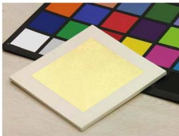
Fig.1 Gold leaf sample used in the experiment.
