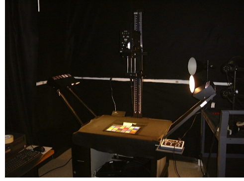
Figure 1: Estimation of pigment concentrations from diffuse spectral reflectance Figure 2: Experimental imaging setup for multiband photometric stereo
