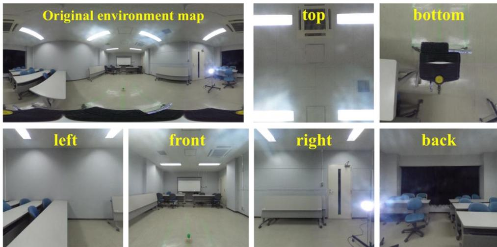
Fig. 5. Environment map and cube map of the image taken in a cuboidal room.
