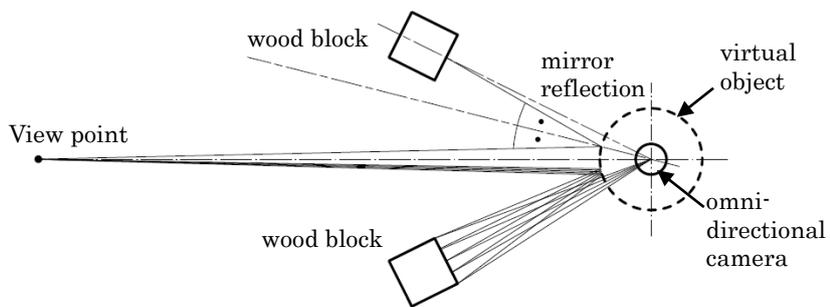
Fig.12 Ray tracing simulation for calculating the actual position of reflection image
