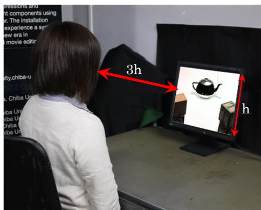
Fig.7 Experimental layout for the symmetrical arrangement
