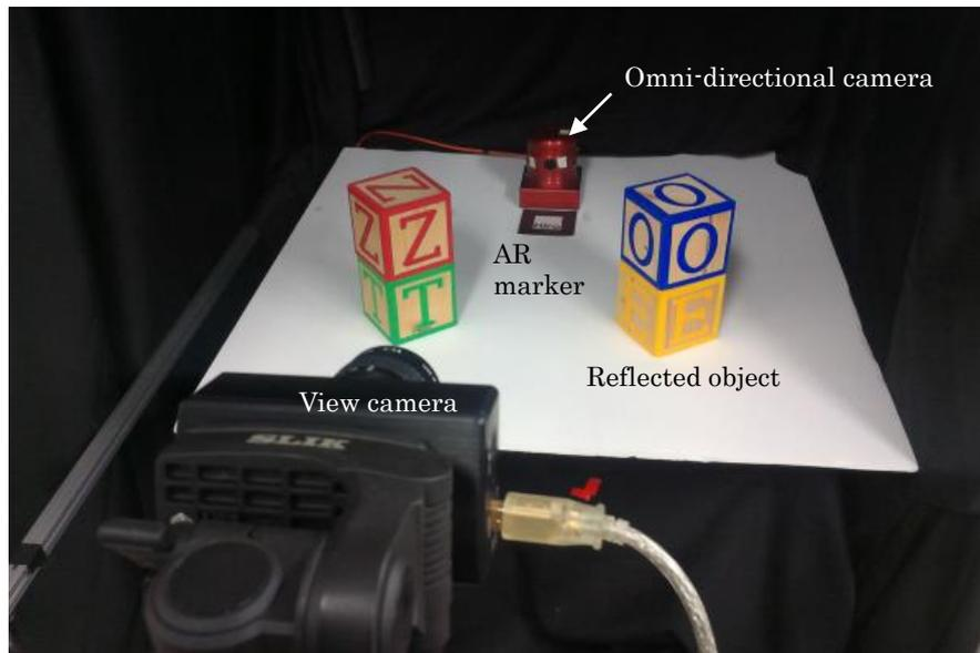
Fig.3 Experimental system for evaluation
