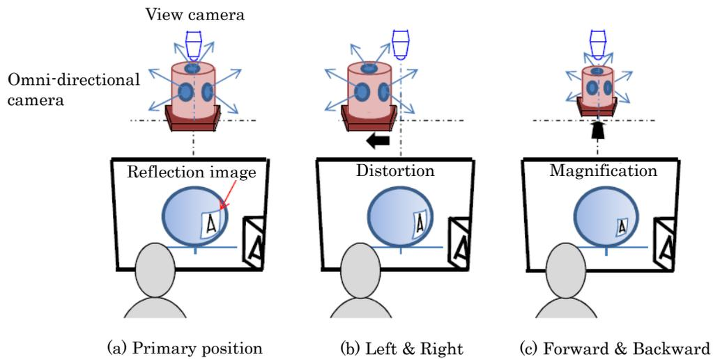
Fig.4 Illustration of reflection images with the change in omnidirectional camera position
