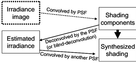
**Figure 2.** Estimation of irradiance by deconvolving the point spread function (PSF) of the medium. The new shading component is simply calculated by convolution between the estimated irradiance and another PSF.
