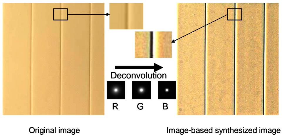
**Figure 5.** The result of deconvolution for the image of the 0.5% phantom by using the PSF measurement
