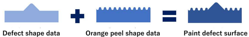
Figure 7. Conceptual diagram of the procedure for generating a paint defect surface.
